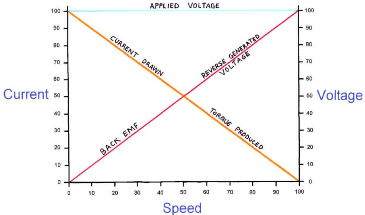
So, here is our boring little drawing again, and now we can see what it really means. The machine is always both a motor and a generator.
