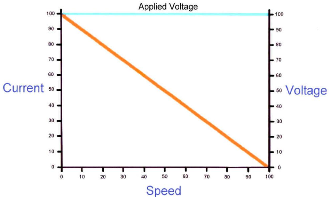
Here is the graph that depicts the torque produced by the machine. With a steady Applied Voltage, the torque produced follows the same characteristics as the Current.
