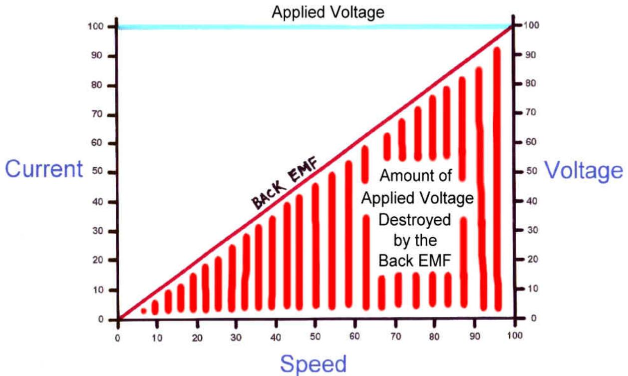
So, just to review, here is a diagram of the Back EMF profile of one of our Permanent Magnet Field DC Motors.
