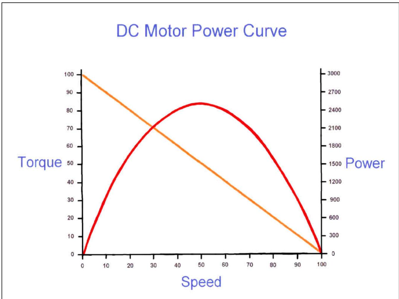
The mechanical energy produced by the machine is seen as the Red Bell Curve.
