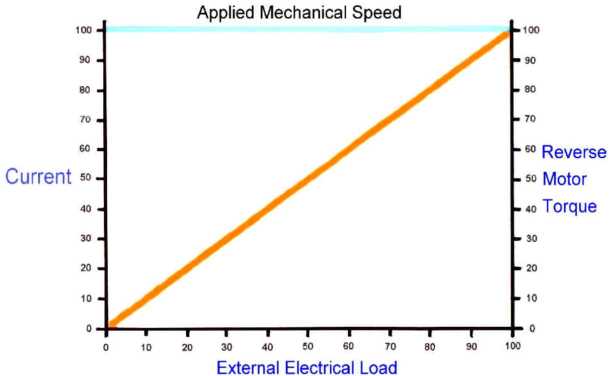
Here is a graph showing the Generator Operations. At any given applied mechanical speed, the production of current to power external loads is in direct proportion to the activation of the reverse motor torque which makes the generator harder to turn.
