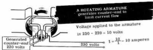
When the motor is just starting and the counter-emf is too small to limit the current effectively, a temporary resistance called the "starting resistance" must be put in series with the armature, to keep the current flow within safe limits. As the motor speeds up, the counter-emf increases and the resistance can be gradually reduced, allowing a further increase in speed and counter-emf. At normal speed, the starting resistance is completely shorted out of the circuit.
