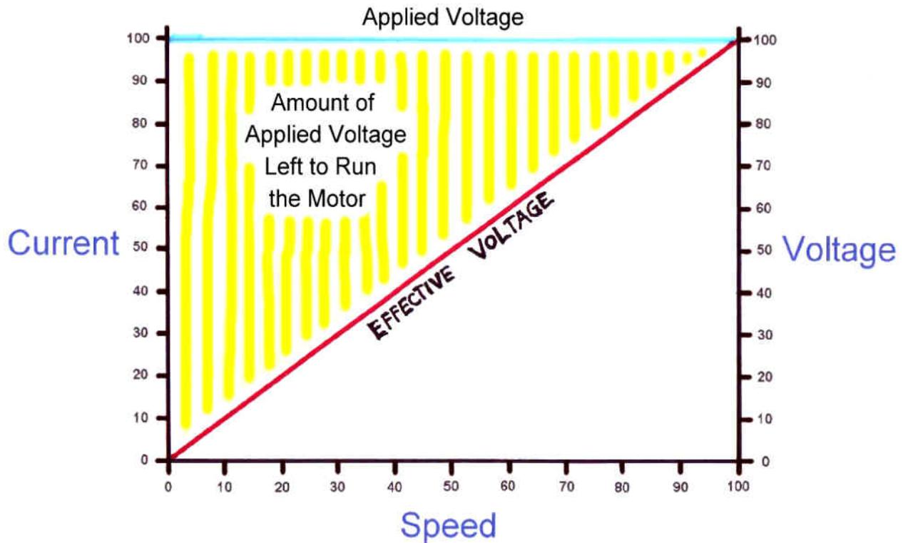
Conversely, this is the diagram that depicts the Effective Voltage Profile. It is what is left when the Back EMF is subtracted from the Applied Voltage.
