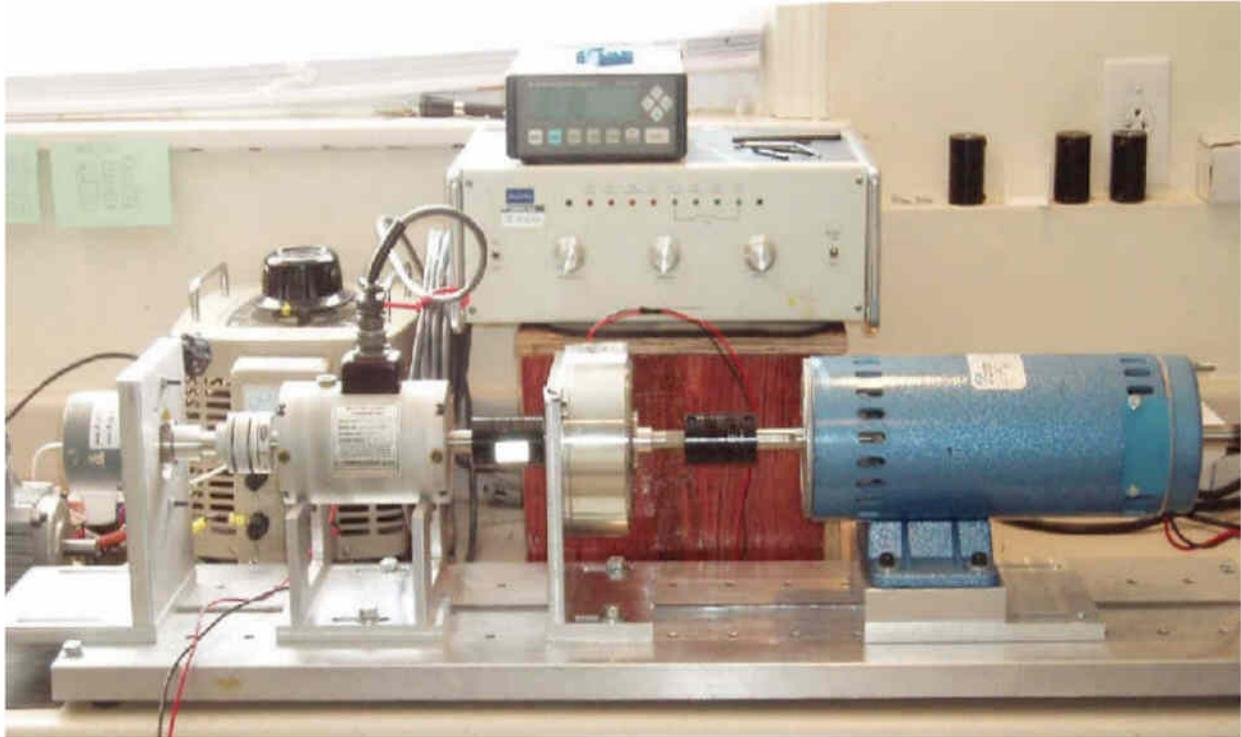
We are told that the best way to determine the efficiency of the machine is just to connect it to an Instrumented Dynamometer and run the test.
