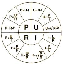
An example of calculating the power consumption of a resistor. Let's say a resistor has a resistance of 10  $\Omega$ , the current passing through the resistor is 1.2 A. The resistor is connected to the load for 1 hour (3600 seconds), let's calculate the work done using the formula (18):
