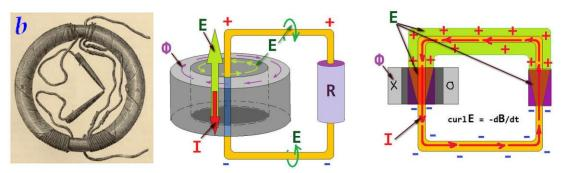
The figure shows the Faraday coil and the principle of operation of the non-contact EMF, which Faraday recorded but unfortunately could not see the difference.
