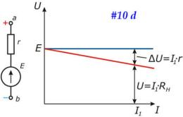
The graph (Fig. #10d) shows the load characteristics of an ideal voltage source (EMF source) (blue line) and a real voltage source (red line).
