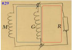
When calculating the generator, we used the circuit marked in red in the figure. We need to find out the possible operation of the circle, which is marked with a blue outline, taking into account the torque of the engine and the electromagnetic moment of the generator.
