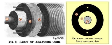
A row of iron rings is attached to a wooden cylinder and shaft by two pins passing through the rings, wooden cylinder and shaft.
