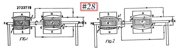
If you are interested, you can read the original patent: <u>https://worldwide.espacenet.com</u> As we look at the drawings from the patent in figure (#28), we see two frame windings, on the same axis, rotating in the magnetic fields of permanent magnets. The frame windings are connected in parallel, and a load R is connected to this connection. On the electrical diagram, it looks very simple and very implausible (Fig. #29).
