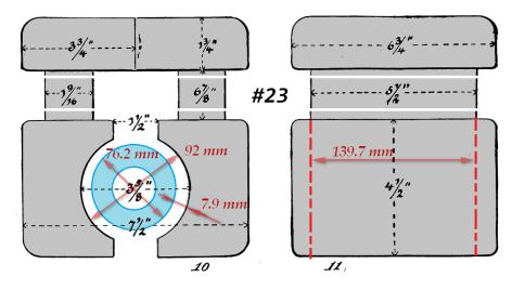
The diameter of the metal ring of the anchor is 76.2 mm; The diameter of the distance between the pole tips is 92.007 mm; The gap between the ring and the pole is 7.9 mm; The length of the anchor that contacts the pole tips is 139.7 mm.
